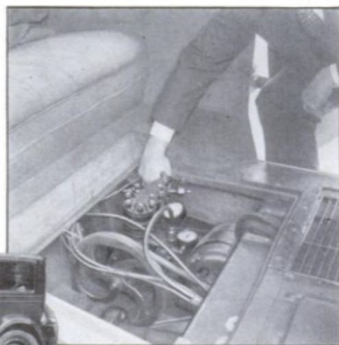
Beneath the floor boards in the auto's rear compartment is placed this refrigerating compressor to chill the air drawn into the car and make driving comfortable on hot days
